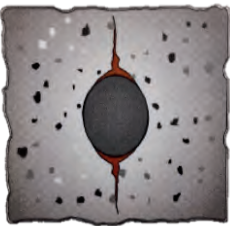
Corrosion starts on the surface of the iron bar
